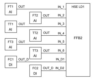
FFB2 is linked to the process devices as shown above. These are the same signals used by FFB1 with the addition of a discrete input from each of the control valves. The discrete input is a Boolean that is true when the valve is closed. There would be contained parameters for the status and alarms in addition to the universal parameters.
