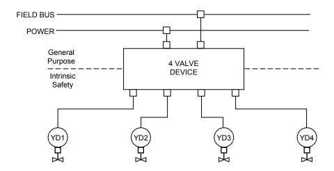
The wiring from the device to the valves may be conventional intrinsically safe multicore cable. It could also be some simple discrete fieldbus suitable to the application. The device contains barrier or other fieldbus hardware.
