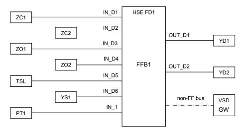
FFB1 is linked to the process devices as shown above. It is shown as a field device FD1 and not as a linking device because it has no H1 ports. The labeled input and output parameters are not linked to any FF device. Instead, the bell wire is hooked to screw terminals on FD1 and the converted values are shown to other FF devices with status in the I/O parameters. The VSD connection is not labeled because it is proprietary, and so is invisible to FF devices.
