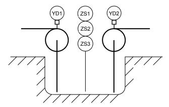
YD1 and YD2 control the two sump pumps. ZS1 closes at the very high level, ZS2 closes at the high level and ZS3 opens when the level drops below the low level setting.
