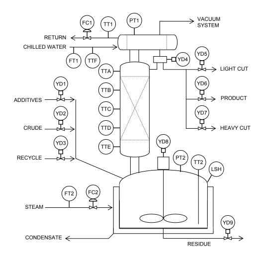
YD1, YD2 and YD3 are block valves for controlling the addition of ingredients.
