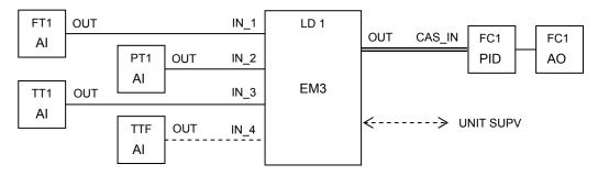
The fourth equipment module is the still pot. It can be set to off, pre-heat, heat to TT2, heat to column pressure drop PT2 minus PT1. The agitator is also controlled through this module.
