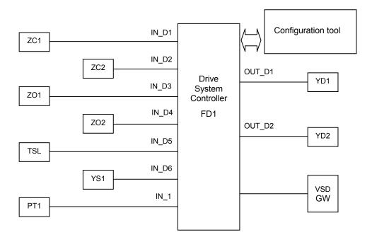
The Drive System Controller is linked to the process devices as shown above. It is shown as a field device FD1 and not as a linking device because it has no H1 ports. The labeled input and output parameters are not linked to any FF device. Instead, the simple sensors are hooked to screw terminals on FD1 and the converted values are shown to other FF devices with status in the parameters of FD1. The VSD connection is not labeled because it is proprietary.
