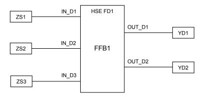
The block uses three of the discrete inputs for the states of Low, High and Very High. It uses two of the discrete outputs for the two pumps. When the Low state is true, both digital outputs are turned off. When the High state becomes true, the previous output remains off and the other output turns on. When the Very High state becomes true, both outputs are turned on and an alarm may be generated.
