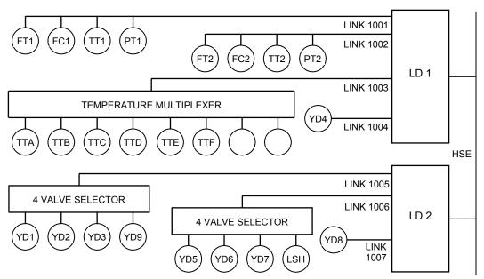
The seven fieldbus cables are connected to two 4-link Batch Linking Devices, so called because they have algorithms for ISA S88 functions, e.g. equipment modules and unit supervision. These connect to HSE fieldbus, which allows communication between linking devices and with the hosts that manage the process and communicate with IT functions.
