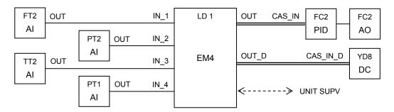
The fifth equipment module contains the column temperature multiplexer and the reflux splitter YD4. The splitter can be set to total reflux, some reflux ratio value, or controlled by a column temperature or the difference between any two column temperatures. The links are made with the Multi-Variable Optimization.
