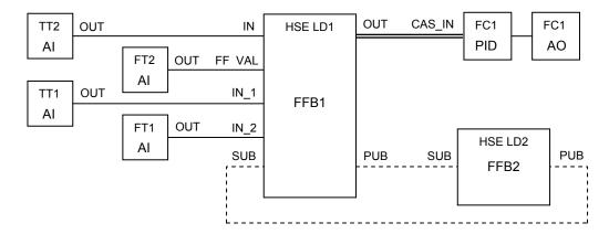
FFB1 is a standard PID with some additional parameters. It behaves like a PID, but it has additional calculations. FFB2 contains calculations that adaptively modify the tuning and feedforward parameters of FFB1 and FFB2 are linked by MVC object lists that are published once during each macrocycle. The additional parameters for FFB1 are listed below, along with the MVC lists.
