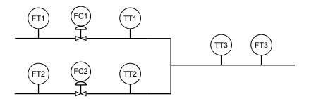
FT1 and FC1 form a loop controlling the associated flow, as does FT2 and FC2. TT1 and TT2 measure the stream temperatures just before they enter the mixing junction and after work done by the valve has changed the temperature. TT3 measures the result of mixing. FT3 is used to determine the amount of heat in the outlet flow.
