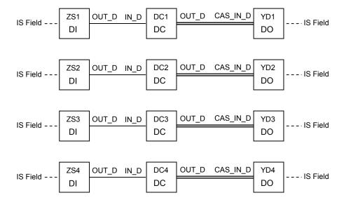
The device contains four instances of a standard discrete control loop, each consisting of a multi-state discrete input for the position sensors, a device control block (see FF-892), and a multi-state discrete output for the actuator. Three state actuators may be used. The twelve blocks share a common OD so that an MVC can contain values from all of them. The MVC list is shown below. There is no FFB, so there is no Block Access list.
